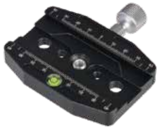
CL-90N Size: 95*90*18mm (3.74*3.54*0.71in) Weight: 130g (0.29lb) Clamp card slot: Arca-Swiss Bottom screw hole: 3/8 "
