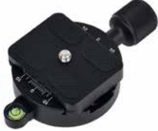
DM-55 Size: 100*55*15mm (3.94*2.17*0.59in) Weight: 110g (0.24lb) Clamp card slot: Arca-Swiss Bottom screw hole: 3/8 "
