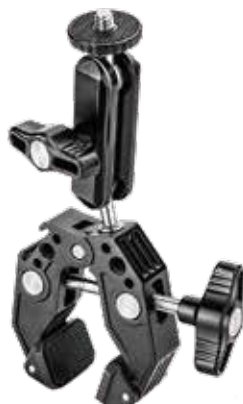
CM-55M Size: 97*88*45mm(3.82*3.46*1.77in) Weight: 200g (0.44lb) Clampable width: 0-2.09in/φ55-φ13 Screw interface: 1/4"
