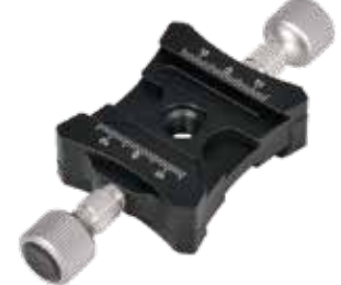
DDR-50 Size: 126*50*20mm (4.96*1.97*0.79in) Weight: 130g (0.29lb) Clamp card slot: Arca-Swiss Bottom screw hole: 3/8 "
