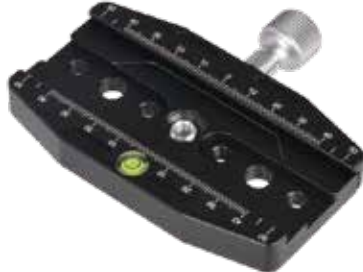
CL-110N Size: 110*95*18mm (4.33*3.74*0.71in) Weight: 168g (0.37lb) Clamp card slot: Arca-Swiss Bottom screw hole: 3/8 "
