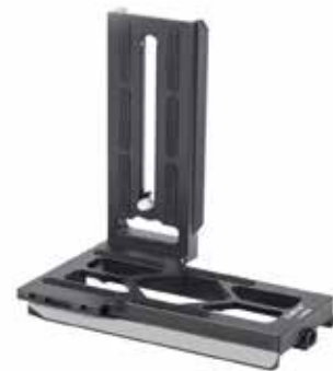
L-QR50 Size: 95*68*120mm(3.74*2.68*4.72in) Weight: 96g (0.21lb) Dovetail groove: Manfrotto/Arca-Swiss QR plate screw: 1/4 "
