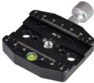
CL-70N Size: 95*70*18mm (3.74*2.76*0.71in) Weight: 110g (0.24lb) Clamp card slot: Arca-Swiss Bottom screw hole: 3/8 "
