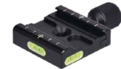
QR-50 Size: 77*50*16mm (3.03*1.97*0.63in) Weight: 90g (0.20lb) Clamp card slot: Arca-Swiss Bottom screw hole: 3/8 "
