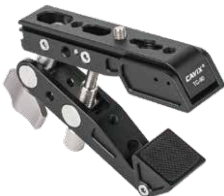
TC-90 Size: 135*31*80mm(5.31*1.22*3.15in) Weight: 250g (0.55lb) Clampable width: 0-2.56in/φ90-φ15 Screw interface: 1/4"
