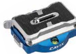
DDR-50 Size: 126*50*20mm (4.96*1.97*0.79in) Weight: 130g (0.29lb) Clamp card slot: Arca-Swiss Bottom screw hole: 3/8 "
