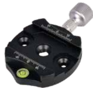
DM-60N Size: 97*60*15mm (3.82*2.36*0.59in) Weight: 88g (0.19lb) Clamp card slot: Arca-Swiss Bottom screw hole: 3/8 "
