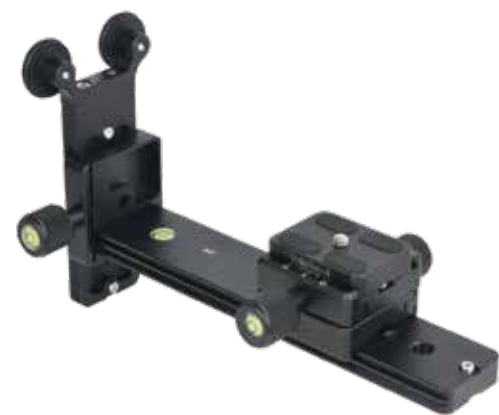
L-200 Size: 220*107*52mm(8.66*4.21*2.05in) Weight: 541g (1.19lb) Load capacity: 15kg(33.07lb) QR Plate model: PU-50 Bottom screw hole: 1/4 " & 3/8 "
