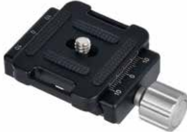
DC-34 Size: 70*44*18mm (2.76*1.73*0.71in) Weight: 70g (0.15lb) Clamp card slot: Arca-Swiss Bottom screw hole: 3/8 "
