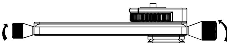
The width of the rail slider is 38mm, user can adjust the slider horizontally with the any of the two supplied fine tuning knobs for precise shooting.
