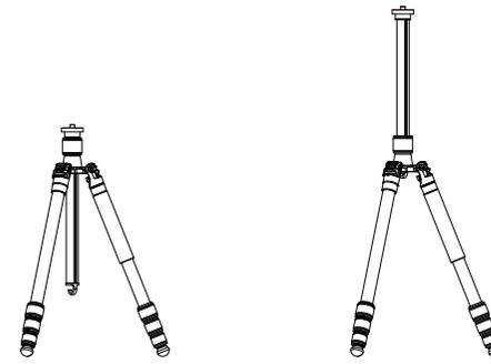
The center column can be adjustable the length by adjustable knob.
