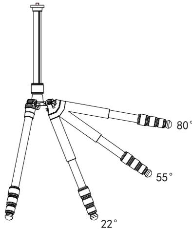
Press the angle adjuster to adjust the angle of the leg, there are three steps of leg angle adjustable, e.g. 80 degree, 55 degree, 22 degree
