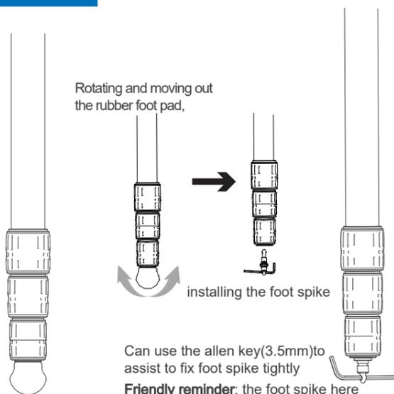
Can use the allen key(3.5mm)to assist to fix foot spike tightly
