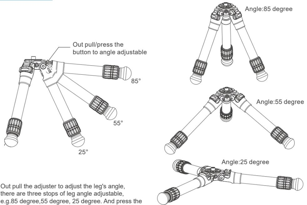
Out pull the adjuster to adjust the leg's angle, there are three stops of leg angle adjustable, e.g. 85 degree, 55 degree, 25 degree. And press the button to lock after angle was adjusted well.
